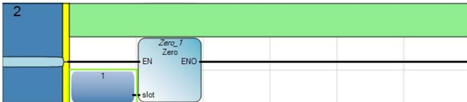
18. To prevent the scale from continuously zeroing, a condition will need to be placed on the rung.
